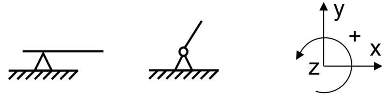
$$\vec{R}_A = \begin{pmatrix} A_x \\ A_y \\ 0 \end{pmatrix} \quad \vec{M}_A = \begin{pmatrix} 0 \\ 0 \\ 0 \end{pmatrix}$$
