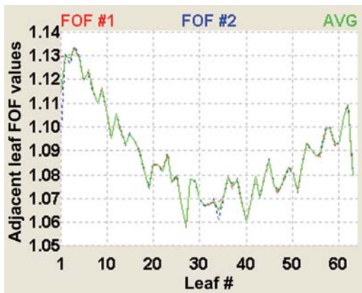
Figure A.2.8. The fluence-output factor (FOF) as a function of leaf number for the TomoTherapy Hi-Art™ system. The measured increase in energy fluence when both neighboring leaves are open is called the FOF. The figure shows the variation in FOF as a function of leaf number. Two runs of the test, listed as FOF1 and FOF2, are shown together with the average results. If only one neighboring leaf is open, the increase in energy fluence is half of the increase shown. The variation from leaf to leaf is due to small (of the order of 25 μm) variations in mechanical precision of the fixture holding the leaves. The asymmetry is due to a lateral offset in the MLC. Calibration of the FOF enables the MLC to operate with wider mechanical tolerances. (Figure courtesy TomoTherapy Inc., Madison, WI, USA; reproduced with permission.)
